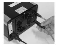
2 In the last light generator a line termination must be mounted in the DMX out.
