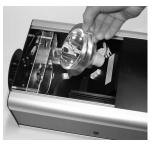
8. install the new lamp in reverse order. Orient the lamp such that the front wire points upwards close to mark.
