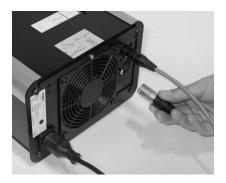
Serial data connection of light generators
