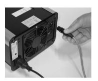
2 If there are more than one light generator they must be connected serially. (See drawing below)
