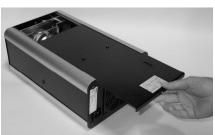
4. Loosen the thumb screw in the lamp bracket.
