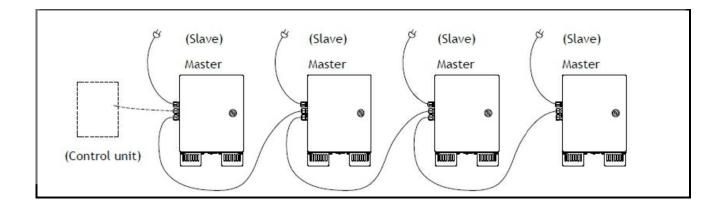
Set the light generator as Master by setting the code wheel 1 to "9".
