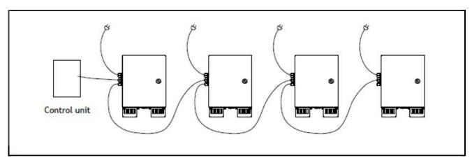
If there is more than one light generator they must be connected in a daisy chain connection.
