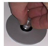
Press in the new reflector
