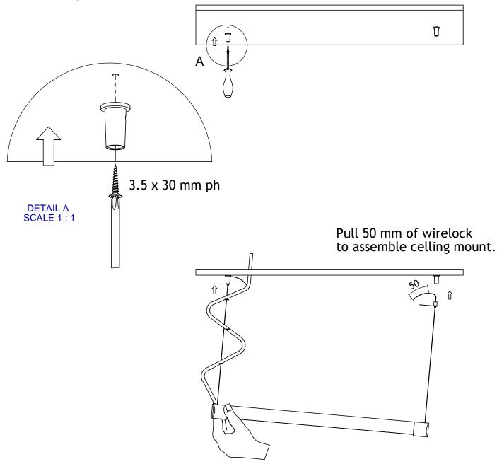
Support fitting while assemble celling mount.
