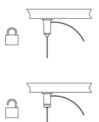
Cut of excess wire close to mounting bracket. Loosend wirelock carefull, pull back /down.
