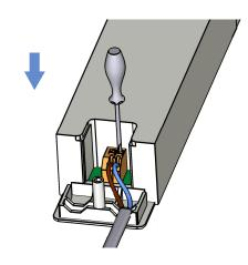
6. Now insert the blue wire in the (L) terminal and the brown wire in the (N) terminal at the other end.
