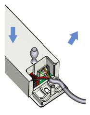
4. To release each wire press the top of the corresponding terminal with a screwdriver. To remove the connector, squeeze the clip on the side and pull
