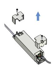
2. Loosen the screws and remove both shields from the driver.
