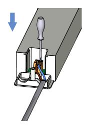
3. To release each wire press the top of the corresponding terminal with a screwdriver
