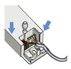
5. To install the new driver, insert the red wire in the + terminal and the blue wire in the - terminal.
