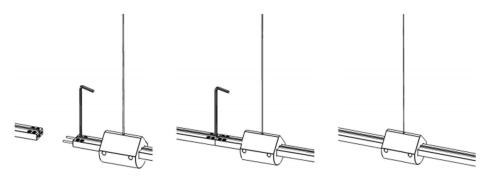
Connect the tracks using the Allenkey and puch the cab to hide the connection.
