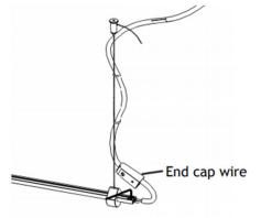
Mount electrical wire trough the End cap.
