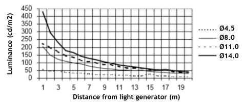
Tested with a 150W light generator. Fibre length: 25 metre, open end. Tested in a Ø0.5 metre Ulbrecht sphere.
